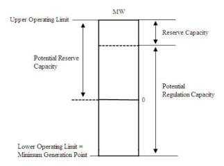
Figure 6: Generating Unit Operating Characteristics
